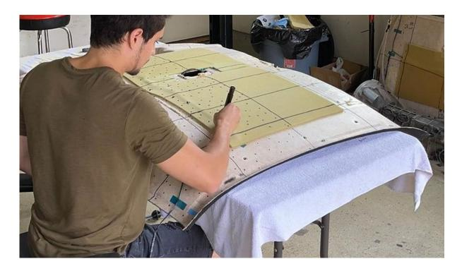
Now that your headliner is detached from your roof and/or removed from your vehicle firstly you want to prepare the module by inserting the fiber batches in to the outputs and then find a suitable location to place the module. (We like to place them at the front, back or centre of the headliner.)
