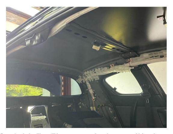
Removing the headliner will be a process somewhat unique to your vehicle, and may require different or specific tools to do so. In general, interior trim pieces like pillar covers, sun visors, map light, dome light and roof handles will need to be removed before the headliner can be detached from the roof, we recommend conducting some research for your specific vehicle to find the process and tools you may need to do so.
